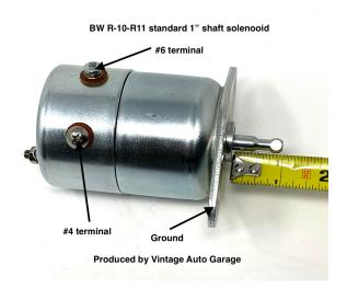
and solenoid, this fools the system and you should hear both relay and solenoid make a clicking sound. When inspecting the solenoid, never press down on the shaft to feel spring tension this can damage and misalign the points inside the solenoid.
